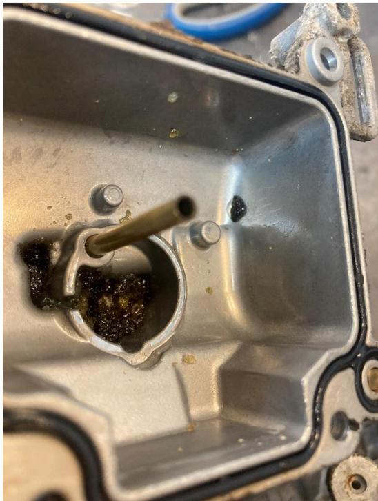
The manual primer pump had also disintegrated so that needed replacing. So, with all jets and floats and internal gubbins stripped apart it all went into the sonic bath in carb cleaning solution for a good 40 minutes at 85°C.
